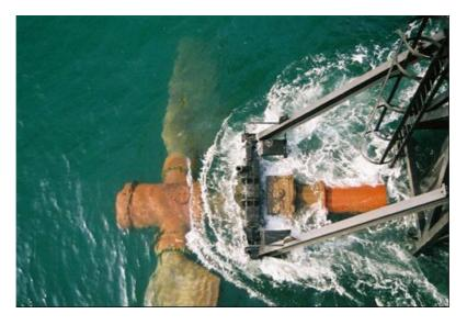
Figure 10. MCT's "Seaflow" tidal stream turbine (brought near surface for maintenance)
