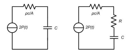
Figure 2. Equivalent electric circuit of tidal behaviour in estuary, without barrage (left) and with barrage (right)
