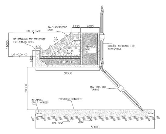
Figure 7. Cross-section of possible concrete caisson
